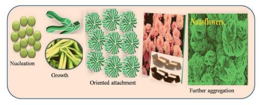
Scheme 1 Plausible mechanism for formation of 3D-nanoflower-like Cu foil coated with CuO (inset: photo image of undeposited and deposited CuO nanoflowers on flexible Cu foil by chemical bath deposition method.
