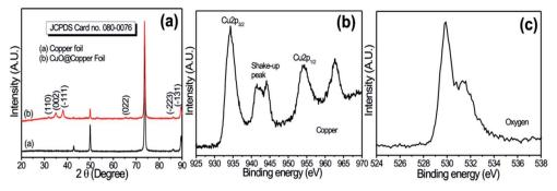
Fig. 1 (a) X-Ray diffraction patterns of copper foil and Cu foil coated with CuO electrode; (b) core-level XPS spectrum of Cu2p; (c) core-level XPS of O1s for CuO samples.
