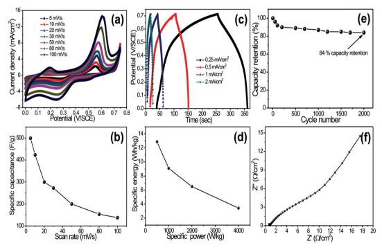
Fig. 4 (a) Cyclic voltammetry (CV) curves at different scanning rates. (b) Variation of specific capacitance with scan rate. (c) Galvanostatic charge—discharge curves at different current densities. (d) Power density *versus* energy density of CuO thin films in a Ragone plot. (e) Plot of percentage capacitance retention with number of cycles. (f) Nyquist plot of CuO-nanoflower-like electrode.
