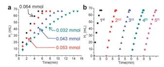
Fig. 4 Plots of volume of hydrogen generated vs. time for catalytic hydrolysis of AB (a) at various concentrations of the Ni@SiO2 catalyst and (b) during the recycling experiment.
