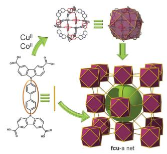
Fig. 12 Linear bridging of the CDC-based MOP by the bent position of the twelve ligands (i.e., using a tetracarboxylate ligand) leads to an SBBbased MOF with fcu topology.
