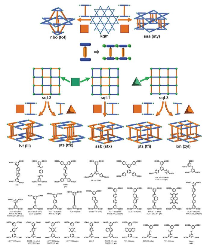
Fig. 30 Schematic of the L-L pillaring of **sql** and **kgm** layers to form the **nbo**, **ssa**, **lvt**, **pts**, **ssb**, and **lon** nets (top), and a non-exhaustive list of ligands that have been used for this type of pillaring (bottom).
