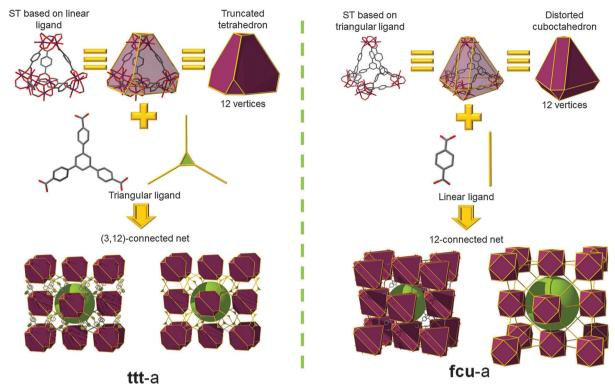
Fig. 7 Topological analysis of MIL-143. Considering the SBBs as truncated tetrahedra constructed from 1,4-BDC and Fe trimers, crosslinked by BTB ligands, the topology is ttt. Considering the SBBs as distorted cuboctahedra constructed from BTB and Fe trimers, bridged by 1,4-BDC ligands, the topology is  ${\it fcu}$  . Both  ${\it fcu}$  and  ${\it ttt}$  are edge-transitive nets.
