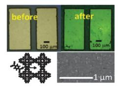
Fig. 35 Optical image of thin MOF film devices before and after TCNQ infiltration (above), schematic of TCNQ molecule entering a HKUST-1 MOF pore, and SEM of the MOF coating (below). Reproduced from Talin et al. 16
