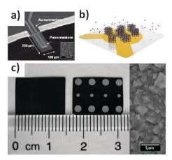
Fig. 31 (a) SEM of piezoresistive microcantilever and inset SEM of MOF deposition (scale bar 2  $\mu$ m), from Allendorf et al.; <sup>264</sup> (b) schematic of the QCM platform (transparent plate) where MOFs are deposited on the gold electrodes (yellow), from Tsotsalas.;55 (c) photograph of HKUST-1 MOF film (left) with Al electrodes attached (right) and SEM image of MOF film surface, from Liu et al.<sup>266</sup>
