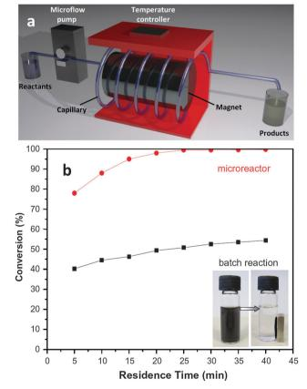
Fig. 25 (a) Schematic of the reactor used for the condensation reaction between benzaldehyde and ethyl cyanoacetate using Fe<sub>3</sub>O<sub>4</sub>@ZIF-8 MFC immobilized along the tube with a magnet; (b) results of the catalytic conversion. The inset shows the fast collection of the composite with an external magnet. From Zhang et al.<sup>216</sup>
