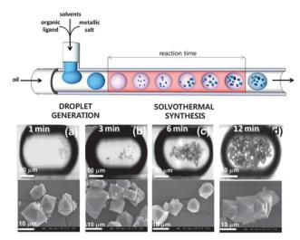
Fig. 15 Schematic representation of a continuous flow microfluidic device for producing high quality MOF crystals (top). Optical and SEM micrographs of HKUST-1 crystals obtained via the microfluidic approach after (a) 1, (b) 3, (c) 6, and (d) 12 min of synthesis. Reproduced from Faustini et al. 150
