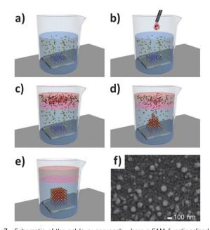
Fig. 7 Schematic of the gel-layer approach where a SAM-functionalised gold substrate is coated with the metal salt gel precursor (a) and then covered in a solution of the organic MOF linker (b). Over time the linker precursor diffuses through the gel to form an oriented MOF crystal (c-e). SEM of NH<sub>2</sub>-MIL-88B(Fe) MOF film formed from the gel layer (f). 49 Video animation provided as ESI.†
