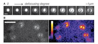
Fig. 3 (A) Transition process from the focused image to the defocused image of H<sub>2</sub>Pc on C18-glass. Laser power: 9.0 μW μm<sup>-2</sup>. Scale bar: 1 μm. Acquisition time for each image: 1.0 s. (B) Defocused images of H<sub>2</sub>Pc at air/ C18-glass interfaces. The image on the right is contrasted and pseudocolored (left images). Scale bar: 5 μm. Laser power: 4.5 μW μm<sup>-2</sup>. Acquisition time for each image: 100 ms
