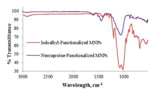
Fig. 2 FR-IR spectra of iodoalkyl-functionalized  $SiO_2$ -coated MNPs **3** and neocuproine-functionalized  $SiO_2$  coated MNPs **7**.
