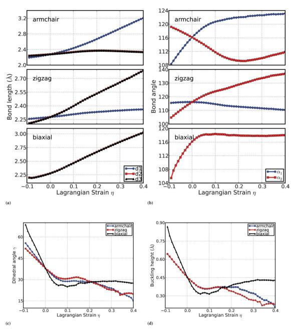
Fig. 3 Evolution of the geometries of b-Si under the armchair, zigzag, and biaxial strains: (a) Bond lengths; (b) Bond angels; (c) Dihedral angles; (d) Buckling height.
