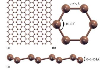
Fig. 1 (a) Silicene plane. (b) Overview and (c) side-view of low-buckled silicene.
