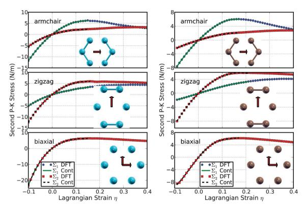
Fig. 5 Stress-strain responses of q-Si (left) and b-Si (right) under the armchair, zigzag, and biaxial strain.  $\Sigma_1$  ( $\Sigma_2$ ) denotes the x (y) component of stress. "Cont" stands for the fitting of DFT calculations ("DFT") to continuum elastic theory. The insets are geometry under ultimate strains.
