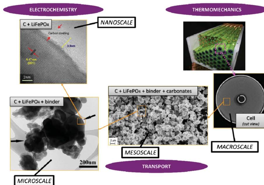
**Fig. 1** Schematics of the multiscale character of a  $\text{LiFePO}_4$  electrode in a LIB and physicochemical mechanisms.<sup>24</sup> Schematics made with TEM and SEM pictures reported in ref. 25 (courtesy of X. Sun, University of Waterloo, Canada) and from the spiral battery tomography picture in ref. 26 (reprinted with permission of Elsevier).
