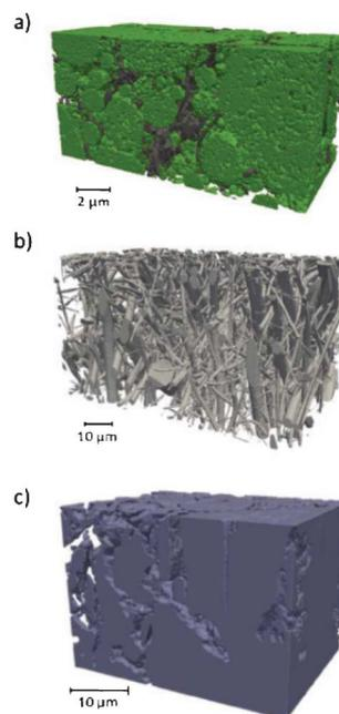
**Fig. 29** 3D reconstructions obtained by FIB tomography of (a) a LiFePO<sub>4</sub> composite positive electrode, (b) a glass fiber separator and (c) a graphite negative electrode. Reprinted with permission from ref. 231. Copyright 2012, The Electrochemical Society.
