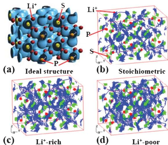
**Fig. 16** (a) the charge density of super cell structure of Li<sub>3</sub>PS<sub>4</sub>. The trajectories of Li<sup>+</sup> ions at 600 K during 36 ps and 90 ps are shown in (b), and (c) to (d), where the concentration of Li is stoichiometric, Li<sup>+</sup>-rich, and Li<sup>+</sup>-poor, respectively. Reprinted with permission from ref. 178. Copyright 2012, The Electrochemical Society.
