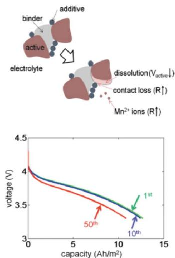
**Fig. 21** top) Schematic diagram of the dissolution process: two  $\text{Mn}^{3+}$  cations convert into one  $\text{Mn}^{4+}$  and one  $\text{Mn}^{2+}$ , then  $\text{Mn}^{2+}$  ions leave the solid phase; down) calculated effect of dissolution and discharge voltage profiles for different numbers of cycles. Reprinted with permission from ref. 206. Copyright 2011, The Electrochemical Society.
