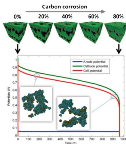
Fig. 39 Multiscale simulation of the PEMFC carbon corrosion by combining a continuum model with a CGMD structural data.<sup>53</sup>
