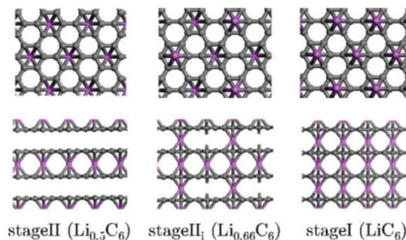
**Fig. 10** Projection views of stage II and stage I crystal structures into the grapheme planes (upper view and along the interlayer direction (lower view)). Lithium atoms are given by large circles on the top of the grapheme layers. Reprinted with permission from ref. 140. Copyright 2008, American Chemical Society.
