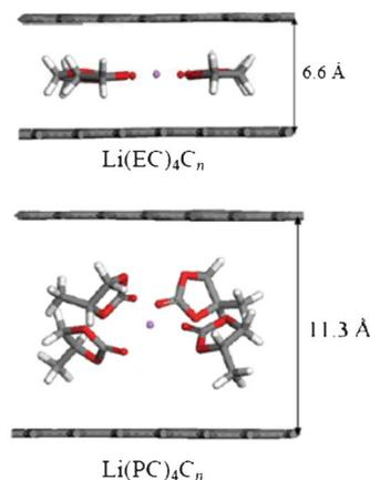
**Fig. 22** the side views of optimized graphene structures with intercalated solvated lithium, calculated by Tasaki *et al.* Reproduced with permission from ref. 215. Copyright 2012, The Electrochemical Society.
