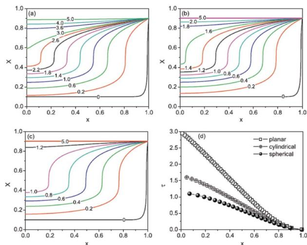
**Fig. 15** Calculated concentration profiles for the dimensionless diffusion equation with phase transformation of the (a) planar, (b) cylindrical, and (c) spherical symmetry. The selected dimensionless times are labelled on the curves. (d) Time dependence of the moving phase boundary. Reprinted from ref. 170 with permission of Elsevier.
