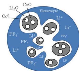
Fig. 11 schematic representation of the most probable electrode morphology, as deduced from the computation of interface energies and energy stress.<sup>141</sup>
