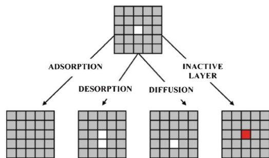
Fig. 18 Schematic representation of the phenomena in the KMC model of Methekar *et al.* Source: 191.
