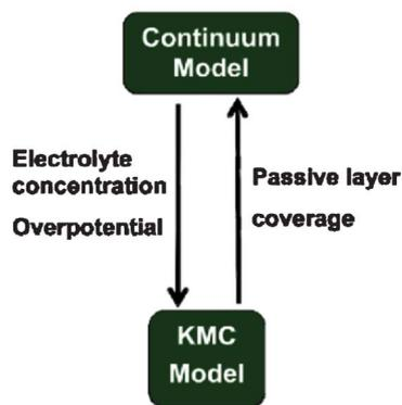
**Fig. 20** Schematics of the coupling of a KMC model with a continuum porous electrode modelling efforts ongoing by Northrop *et al.* Reproduced with permission from ref. 193. Copyright 2012, The Electrochemical Society.
