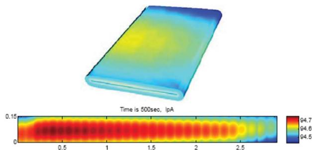
**Fig. 36** Reaction current density distribution after 500 s at 4C discharge of 20 Ah cell with continuous tabs at (a) surface and (b) unrolled jelly roll. Reproduced with permission from ref. 262. Copyright 2012, The Electrochemical Society.
