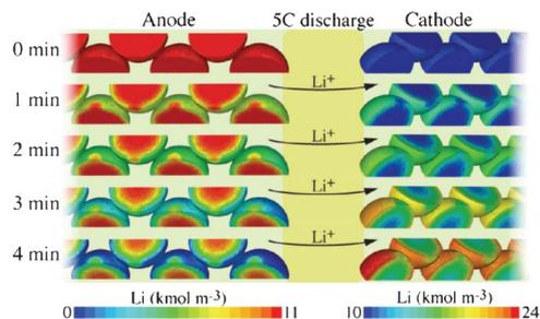
**Fig. 25** Calculated Li concentration within the electrode particles during a 5C discharge. Reprinted from ref. 220 with permission of Elsevier.
