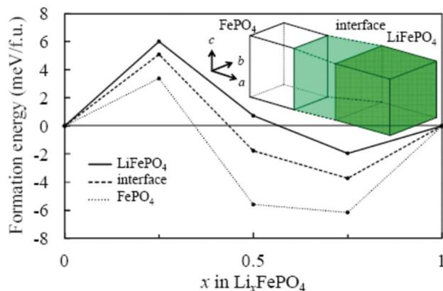
**Fig. 8** Calculated formation energy of solid-solution phase of olivine-type  $\text{Li}_x\text{FePO}_4$  by Asari *et al.* Solid, broken and dotted lines indicate lithiated, interface, and delithiated regions respectively. Reprinted with permission from ref. 135. Copyright 2012, The Electrochemical Society.
