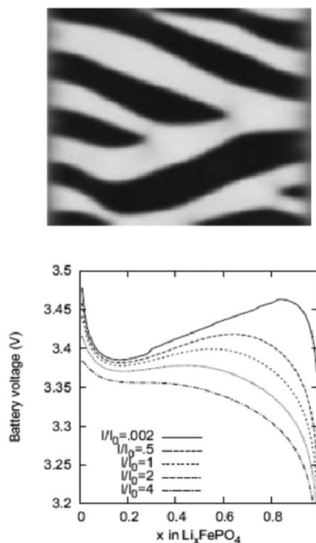
**Fig. 14** Top) calculated phase separation in a particle which has been allowed to relax from a homogeneous state at zero current with stress-free boundaries. White regions are lithium-rich. Down) Calculated LIB voltage at different applied currents. Reprinted with permission from ref. 169. Copyright 2011, The Electrochemical Society.
