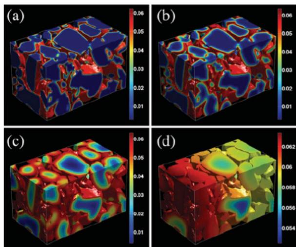
**Fig. 30** Li concentration ( $\text{mol cm}^{-3}$ ) evolution during the discharge of a  $\text{Li}_x\text{CoO}_2$  microstructure at a constant voltage loading. Through electrochemical reaction, Li ions are injected into cathode particles: (a)–(d) corresponding to time of 4.04, 20.1, 133.3 and 1226.5 s (assuming the value of the diffusion coefficient of  $10^{-10} \text{ cm}^2 \text{ s}^{-1}$ ). Reprinted with permission from ref. 234. Copyright 2012, The Electrochemical Society.
