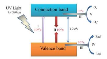
**Fig. 1** Primary steps in the photocatalytic mechanism (TiO<sub>2</sub>): (I) formation of electron (e<sup>-</sup>)-hole (h<sup>+</sup>) pairs by photoexcitation; (II) photoinduced charge recombination; (III) photoinduced charge transportation; (IV) oxidation caused by a valence band hole; (V) reduction caused by a conduction band electron (adapted with permission from ref. 3, copyright 1995 American Chemical Society).
