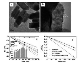
Fig. 13 The morphology of ZnWO<sub>4</sub> and C<sub>3</sub>N<sub>4</sub>/ZnWO<sub>4</sub> photocatalysts: (a) ZnWO<sub>4</sub> (b) C<sub>3</sub>N<sub>4</sub>/ZnWO<sub>4</sub>; pseudo-first-order rates of MB degradation over  $ZnWO_4$  and  $C_3N_4/ZnWO_4$  photocatalysts: (c) under UV light irradiation ( $\lambda =$ 254 nm) (d) under visible light irradiation ( $\lambda > 420$  nm) (reprinted with permission from ref. 26, copyright 2012 Royal Society of Chemistry).
