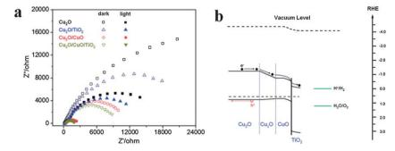
Fig. 15 (a) EIS data of Cu<sub>2</sub>O, Cu<sub>2</sub>O/CuO and Cu<sub>2</sub>O/CuO/TiO<sub>2</sub> nanowire array based photocathodes both in the dark and under light; (b) energy band diagram and charge transfer for Cu<sub>2</sub>O/CuO/TiO<sub>2</sub> (reprinted with permission from ref. 117, copyright 2013 Royal Society of Chemistry).
