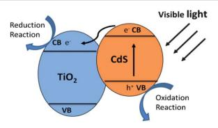
Fig. 9 Schematic illustration of charge transfer in CdS/TiO<sub>2</sub> heterostructure.
