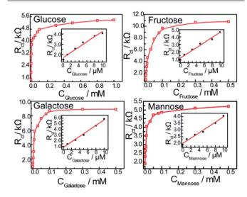
**Fig. 5** Calibration curves obtained using  $R_{\rm ct}$  as a function of saccharide concentration. The frequency range is between 100 mHz and 100 kHz at the half-wave potential of 0.20 V with 10 mV sine wave potential. The inset shows the linear relationship between the  $R_{\rm ct}$  and the concentration of saccharides (from 0 to 10  $\mu$ M).
