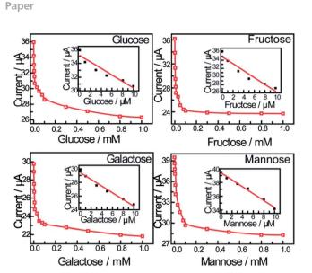
**Fig. 3** The calibration curve obtained using peak current as a function of saccharide concentration. The inset shows the linear relationship between the peak current and the concentration of saccharides applied in the calibration (from 0 to 10  $\mu$ M).
