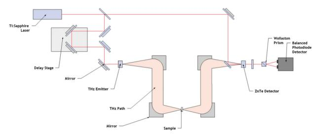
Fig. 7 Schematic representation of a common Terahertz Time Domain Spectroscopy System.
