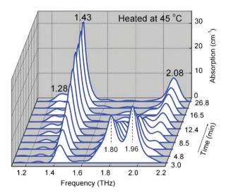
**Fig. 6** THz absorption spectra (with baselines corrected) of p-glucose monohydrate being heated at 45 °C for about 27 min. The numbers mark the positions of absorption peaks. The absorption peaks at 1.80 and 1.96 THz decreased and the absorption peaks at 1.28, 1.43, and 2.08 THz increased over time due to the reduction of p-glucose monohydrate and augment of anhydrous p-glucose during the dehydration. (Reproduced with permission of Elsevier from ref. 47).
