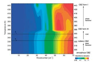
**Fig. 4** Contour plot of the non-isothermal heating of amorphous carbamazepine (CBZ) from room temperature. The sample was heated from 293 K until its melting point at a heating rate of 1 K min<sup>-1</sup>. (Reproduced with permission of John Wiley & Sons, Inc. from ref. 42.)
