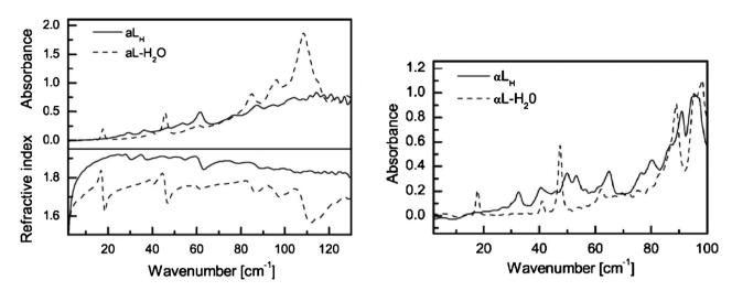
Fig. 3 Terahertz absorption spectra and frequency dependent refractive indices of  $\alpha$ -lactose anhydrate (aL<sub>H</sub>) and  $\alpha$ -lactose monohydrate (aL-H<sub>2</sub>O) at 293 K (left) and 90 K (right). (Reproduced with permission of Elsevier from ref. 14).
