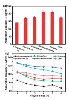
**Fig. 5** (a) Oil and organic solvent absorption capacities of the graphene–CNT hybrid foams. The error bars indicate the standard deviations from 3 samples. (b) Absorption recyclability of the graphene–CNT hybrid foams for oils and organic solvents.
