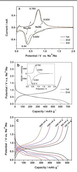
**Fig. 2** Electrochemical properties of the Sb/C nanocomposite: (a) The CV curve at a scan rate of 0.1 mV s<sup>-1</sup> ( $\nu s$ . Na<sup>+</sup>/Na); (b) charge–discharge curves of the Sb/C composite at a constant current of 100 mA g<sup>-1</sup>, the inset is differential capacity *versus* cell potential curve; (c) charge–discharge profiles at various current densities from 150 mA g<sup>-1</sup> to 2000 mA g<sup>-1</sup>.
