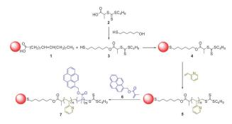
Scheme 1 Synthesis of (PyMMP-b-P2VP)-CdSe/ZnS QDs.
