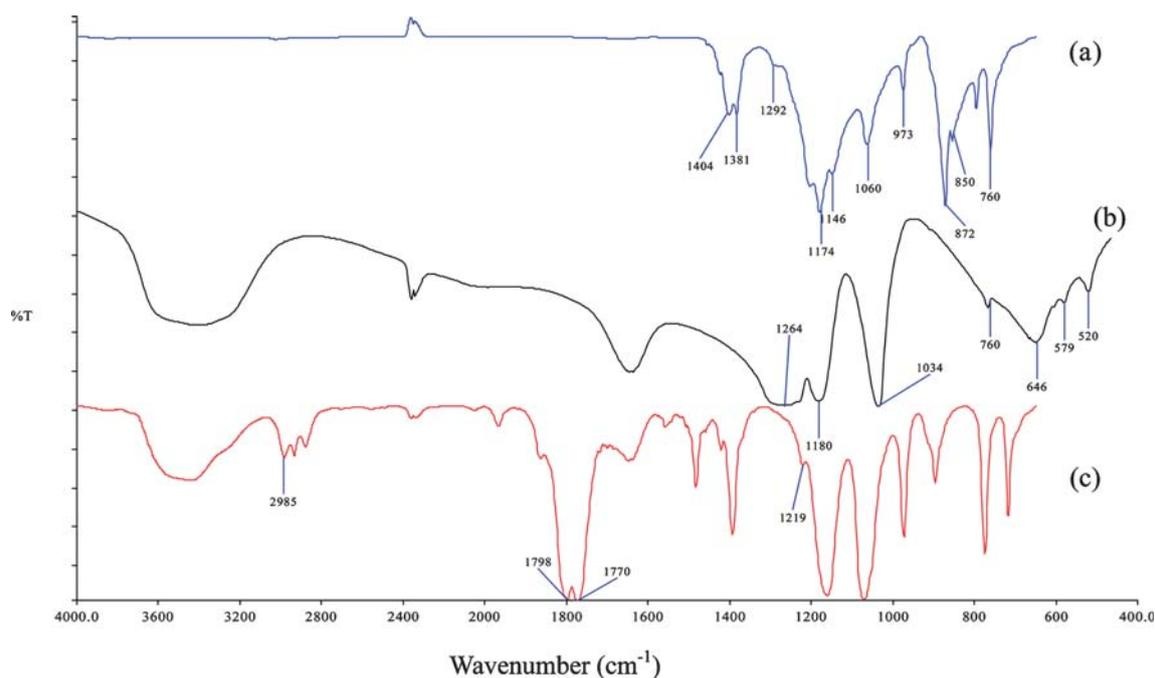
Fig. 7 The FTIR spectra for (a) pure PVdF-HFP; (b) pure LITf; (c) pure EC.
