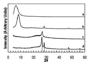
**Fig. 2** X-Ray diffraction patterns of: (a) GO paper; (b) SGO paper; (c) graphene paper by reduction of GO paper; (d) SG paper by reduction of SGO. Diffractions due to graphite (26.4°) and Si (111), (220), and (311) at 28.3°, 47.2°, and 56.1°, respectively, are indicated.
