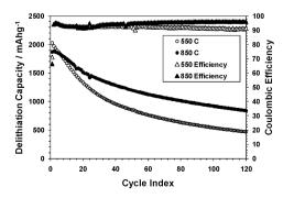
**Fig. 4** Delithiation capacities and coulomb efficiencies of SG samples reduced at 550 or 850 °C, using a constant current–constant voltage (CCCV) method (1.5–0.020 V, 1000–50 mA g $^{-1}$ ).
