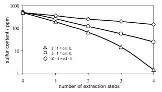
**Fig. 1** Multistage desulfurization of model diesel oil (500 ppm sulfur in ndodecane) by the IL [BMIM]Cl/AlCl<sub>3</sub> (0.35/0.65; different mass ratios oil/IL) at room temperature.
