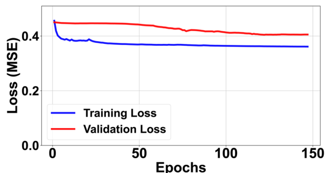
Fig. 1 Learning dynamics for the autoencoder trained on standardised descriptors. Training and validation MSE drop rapidly and then evolve into a broad, stable plateau without divergence, indicating that the model has reached a regime of stable compression without strong overfitting. The vertical axis starts at zero to show the full loss scale. Final losses: training 0.3204, validation 0.3954.
