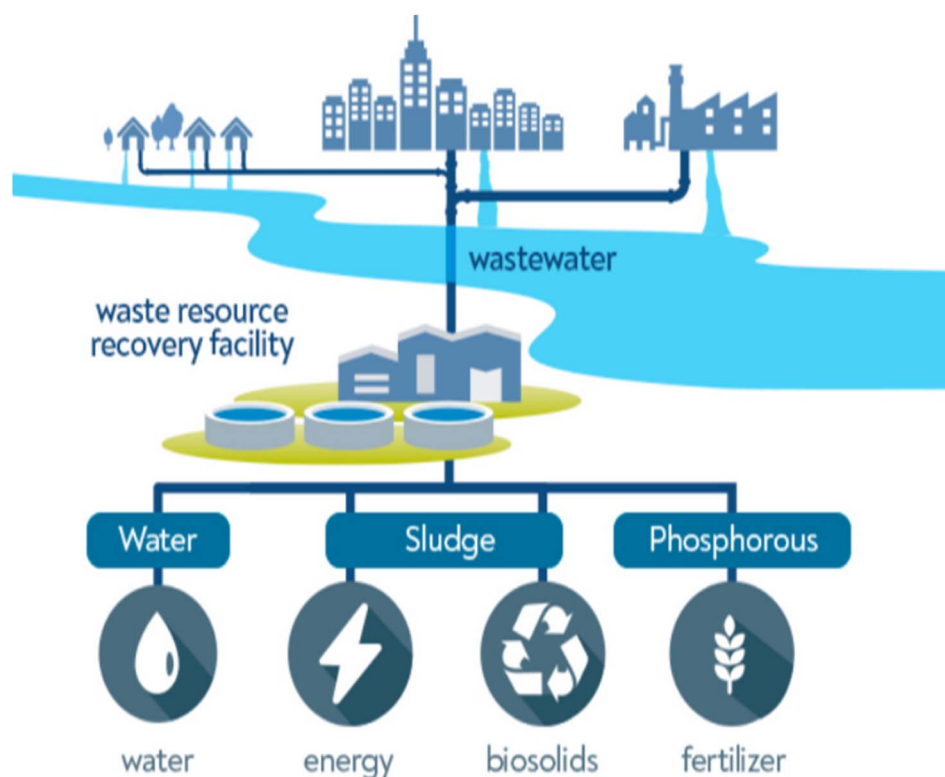
Fig. 1 Stages and applications of wastewater treatment (ref. 36).
