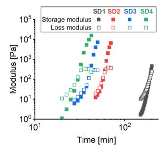
Fig. 2 Time sweep rheological analysis of the pre-gel mixtures SD 1 to SD 4.
