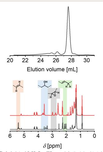
Fig. 1 Analysis of EpCO. Top: SEC curves (refractive index detector). Bottom: Overlay of proton nuclear magnetic spectra of CO (black) and EpCO (red), and assignments of peaks related to epoxidation.
