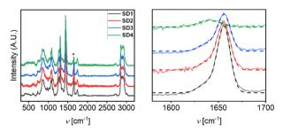
Fig. 3 RAMAN analysis of the cured SD 1 to SD 4 gels. Left: Traces overlay. Right zoom in in the region between 1580 and 1700 cm<sup>-1</sup> of the RAMAN curves (full lines) related to both C=C and oxazolidone stretching frequencies and fitting according to Gaussian extrapolation (peaks at 1640 and 1656 cm<sup>-1</sup>, dotted lines).
