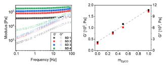
Fig. 6 Rheological analysis of samples SD 1 to SD 4. Left: Frequency sweep curves of gels. Right: Plot of G' and G'' at 1 Hz vs. mass fraction of EpCO over CO; the dotted line is a guide.
