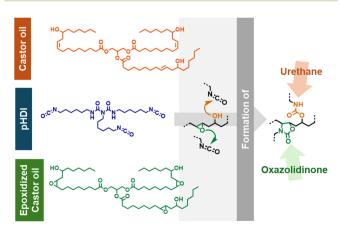
Scheme 1 Representation of the reaction between CO, EpCO and pHDI (poly(hexamethylene diisocyanate)).
