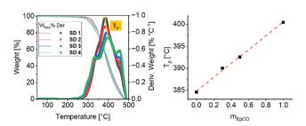
Fig. 5 TGA analysis of the SD 1 to SD 4 samples. Left: Weight loss (line) and derivative weight loss curves (dots) and depiction of the derivative peak temperature ( $T_p$ ) of the more intense degradation step. Right: Evolution of  $T_p$  over mass fraction of EpCO over CO; the dotted line is a
