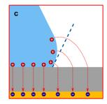
Fig. 4 (a) A sliding drop affected by electrostatic contact angle hysteresis, electrowetting, and electric breakdown. (b) and (c) Details of the electric fields causing Maxwell stress on the drop in the case of electrostatic contact angle hysteresis (b) and electrowetting (c).
