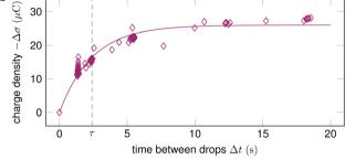
Fig. 3 (a) The drop charge at a fixed position x along the slide path decreases and then saturates with increasing drop number. Data reproduced from ref. 19; (b) By varying the time between drops  $\Delta t$  and measuring the change in surface charge density  $\Delta \sigma$ , the characteristic discharge time  $\tau$  can be quantified. Data reproduced from ref. 32.
