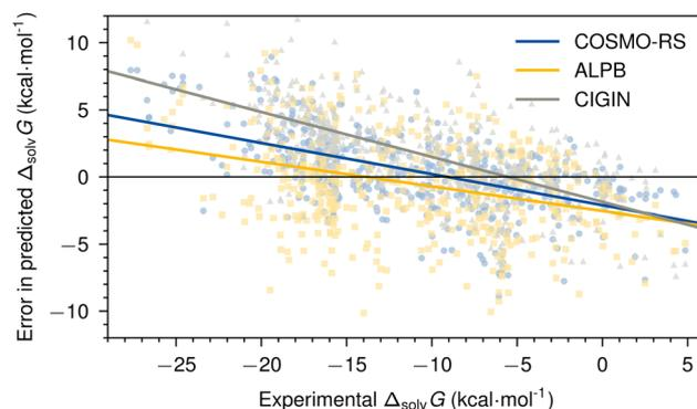
Fig. 7 Error in computed solvation energy ( $\Delta_{\text{solv}}G$ ) versus experimental  $\Delta_{\text{solv}}G$  for three representative models: COSMO-RS (QM, blue circles), ALPB (SQM, yellow squares), and CIGIN (ML, gray triangles). Solid lines show linear regression lines of the errors, indicating each model's systematic underestimation of large (positive) and overestimation of small (negative) values. All values are given in kcal mol<sup>-1</sup>.
