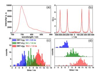
Fig. 3 (a) Fluorescence spectrum of a single  $DBT\_d_{20}$  molecule in Zeonex. (b) Coincidence count rate  $C(\tau)$  after pulsed excitation of a single  $DBT\_d_{20}$  molecule at room temperature. (c) Single molecule fluorescence lifetime distributions of  $DBT\_h_{20}$  (blue),  $DBT\_h_{12}$  (green) and  $DBT\_d_{20}$  (red) in Zeonex. In (d) the distributions are plotted separately for clarity.
