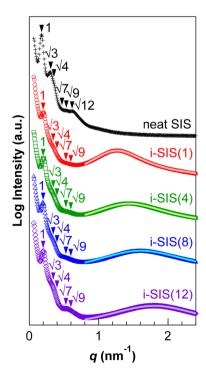
**Fig. 6** SAXS profiles of neat SIS (black plus marks), i-SIS(1) (red open circles), i-SIS(4) (green open squares), i-SIS(8) (blue open triangles), and i-SIS(12) (purple open diamonds). The light-colored solid lines over the profiles of i-SIS(*n*) represent fitting curves based on the Yarusso–Cooper model.
