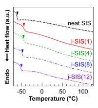
Fig. 4 DSC thermograms of neat SIS (black dotted line), i-SIS(1) (red solid line), i-SIS(4) (green dashed line), i-SIS(8) (blue dashed-dotted line), and i-SIS(12) (purple dashed-two-dotted line). Arrows indicate the positions of  $T_{\rm q}$  of the middle block.
