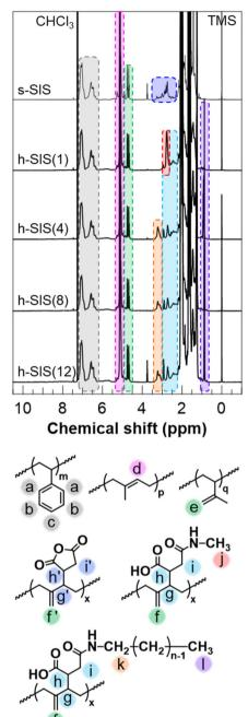
Fig. 2 <sup>1</sup>H NMR spectra of s-SIS, h-SIS(1), h-SIS(4), h-SIS(8) and h-SIS (12), and chemical structures of polystyrene, poly(1,4-isoprene), poly (3,4-isoprene), succinic anhydride incorporated-poly(1,4-isoprene), and hydrogen bonding group-incorporated poly(1,4-isoprene), where chemical structures of other isomers are omitted for simplicity.
