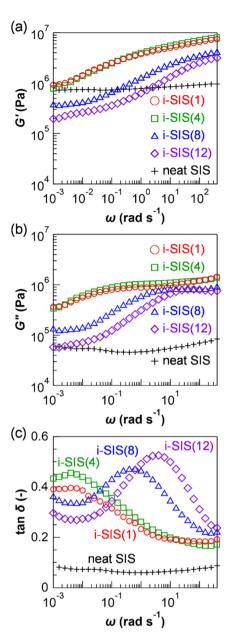
Fig. 7 Frequency dependence of (a) storage moduli, G', (b) loss moduli, G'', and (c)  $\tan \delta$  acquired by dynamic mechanical tests at room temperature for neat SIS (black plus marks), i-SIS(1) (red open circles), i-SIS(4) (green open squares), i-SIS(8) (blue open triangles), and i-SIS(12) (purple open diamonds).
