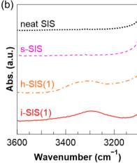
Fig. 3 FT-IR spectra of neat SIS (black dotted line), s-SIS (pink dashed line), h-SIS(1) (orange dashed-dotted line), and i-SIS(1) (red solid line) within the wavenumber ranges of (a) 1500 to 2000  $\rm cm^{-1}$  and (b) 3100 to 3600  $\rm cm^{-1}$ .
