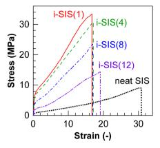
Fig. 9 Typical tensile stress-strain curves of neat SIS (black dotted line), i-SIS(1) (red solid line), i-SIS(4) (green dashed line), i-SIS(8) (blue dashed-dotted line), and i-SIS(12) (purple dashed-two-dotted line).
