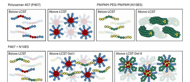
Fig. 3 Proposed gelation mechanism for P407, N10E5, and the P407 + N10E5 composite gel. For P407, blue circles represent PEO and red circles represent the PPO blocks. For N10E5, NIPAM is shown as yellow circles and PEG as green circles.
