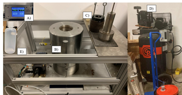
Fig. 11 Pressure BioSciences Inc. pilot scale high pressure reactor indicating (A) pressure indicator, (B) 5 L chamber, (C) screw cap, (D) air compressor, (E) 1000 mL LDPE reaction bottle.
