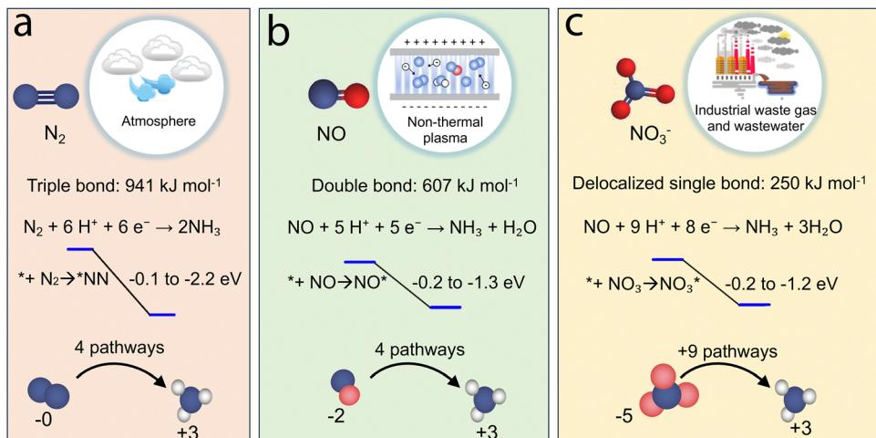
Fig. 2 Electroreduction pathways for ammonia synthesis from nitrogen species at different oxidation states, (a) N<sub>2</sub> (0), (b) NO (+2), and (c) NO<sub>3</sub><sup>-</sup> (+5), along with their respective sources, bond dissociation energies (kJ mol<sup>-1</sup>), overall reduction stoichiometries, and first-step adsorption free energies. Sphere colours denote nitrogen (blue), oxygen (red), and hydrogen (white).
