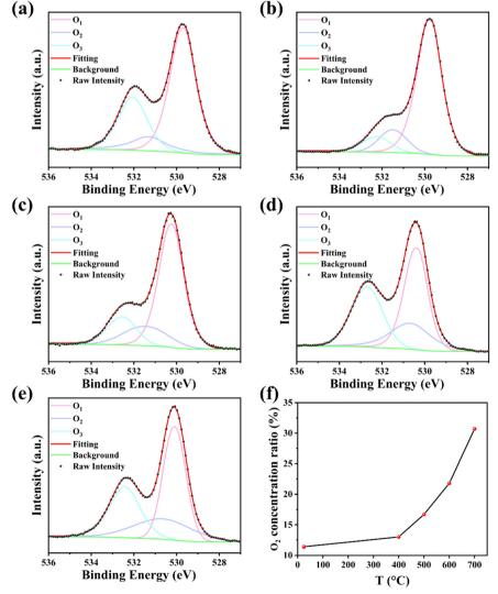
Fig. 5 (a) The O 1s electron spectra of LiNbO<sub>3</sub> wafers untreated at 25 °C and treated at different reduction temperatures: (b) 400 °C, (c) 500 °C, (d) 600 °C, and (e) 700 °C, fitted using a Gaussian-Lorentzian mixed function. (f) Plot of the O2 concentration ratio on the surface of LiNbO3 crystals untreated at 25 °C and treated at different reduction temperatures (400 °C, 500 °C, 600 °C, and 700 °C).
