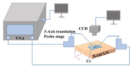
Fig. 1 Schematic diagram of S-parameter measurement of lithium niobate-on-wafer devices
