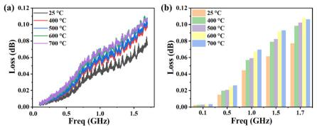
Fig. 6 (a) The relationship between the substrate loss of on-chip  $LiNbO_3$  devices and frequency in the range of 0.1 to 1.7 GHz for untreated and treated samples at different reduction temperatures. (b) The substrate loss of on-chip  $LiNbO_3$  devices at frequency points of 0.1 GHz, 0.5 GHz, 1.0 GHz, 1.5 GHz, and 1.7 GHz for untreated and treated samples at different reduction temperatures.
