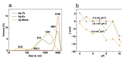
Fig. 4 Crystal size distribution in volume (a) and  $\zeta$ -potential vs. pH (b) of the samples Ap blank (orange), Ap-Eu (red) and Ap-Tb (green line) prepared at 200 °C in presence of 10 mM lanthanide.
