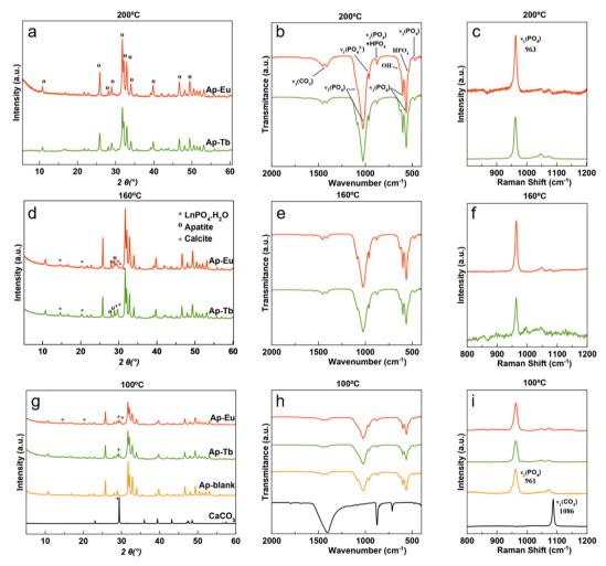
Fig. 1 Conversion of bCC powder to Ap-Eu and Ap-Tb particles at 100, 160 and 200 °C for 7 days analyzed by XRD (a, d and g), FTIR spectroscopy (b, e and h) and Raman spectroscopy (c, f and i).
