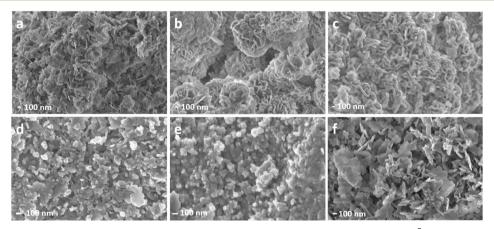
Fig. 2 VPSEM micrographs of Ap–Eu and Ap–Tb samples prepared at 160 °C in the presence of 10 mM of Eu<sup>3+</sup> (a) and 10 mM Tb<sup>3+</sup> (d), at 200 °C in the presence of 10 mM Eu<sup>3+</sup> (b) and 10 mM Tb<sup>3+</sup> (e), and at 200 °C in the presence of 20 mM Eu<sup>3+</sup> (c) and 20 mM Tb<sup>3+</sup> (f).
