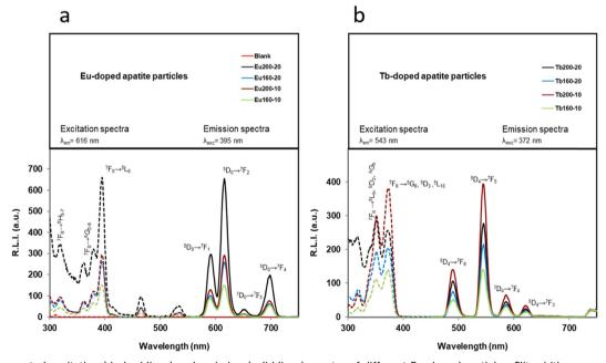
Fig. 5 (a) Uncorrected excitation (dashed lines) and emission (solid lines) spectra of different Eu-doped particles. Slit-width<sub>exc/em</sub> = 10/10 nm,  $t_d$  = 120  $\mu$ s,  $t_g$  = 5 ms and voltage detector = 530 V. (b) Uncorrected excitation (dashed lines) and emission (solid lines) spectra of the Tb-doped particles. Slit-widths<sub>exc/em</sub> = 10/10 nm,  $t_d$  = 120  $\mu$ s,  $t_g$  = 5 ms and voltage detector = 580 V.
