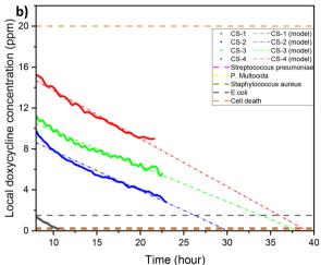
Fig. 5 a) Release profiles for CS-4, CS-3, CS-2, CS-1 over a 24 hour period, b) linear best fit line for release profiles to completion, pH 5.5, 37 °C cross sectional area of 7 mm<sup>2</sup>, depth of 0.5 mm, and 10 μL volume, unstimulated flow.
