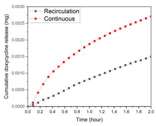
Fig. 10 Release profile for CS-2 under stimulated flow continuous flow and re-circulatory flow, pH 5.5, 37  $^{\circ}$ C cross sectional area of 7 mm², depth of 0.5 mm, and 10  $\mu$ L volume.
