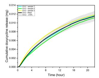
Fig. 4 Repeatability test in the microfluidic device. Three identical samples were tested, and the deviation of final drug concentration was less than 5%, pH 5.5, 37 °C cross sectional area of 7 mm², depth of 0.5 mm, and 10  $\mu$ L volume, unstimulated flow.
