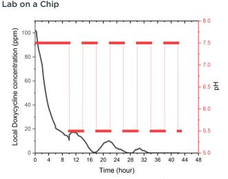
Fig. 9 Release profile for 3 (wt)% and 40 mg mL $^{-1}$  doxycycline loaded scaffold exposed to pH pulses, cross sectional area of 7 mm $^2$ , pH 5.5 and 7.5, 37 °C cross sectional area of 7 mm $^2$ , depth of 0.5 mm, and 10  $\mu$ L volume, unstimulated flow.
