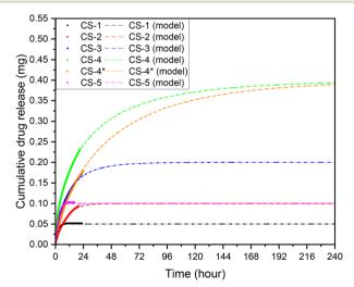
Fig. 7 Weibull models for; CS-1, CS-2, CS-3, CS-4, CS-5, CS-4\* pH 5.5, 37 °C cross sectional area of 7 mm<sup>2</sup>, depth of 0.5 mm, and 10 μL volume, unstimulated flow.
