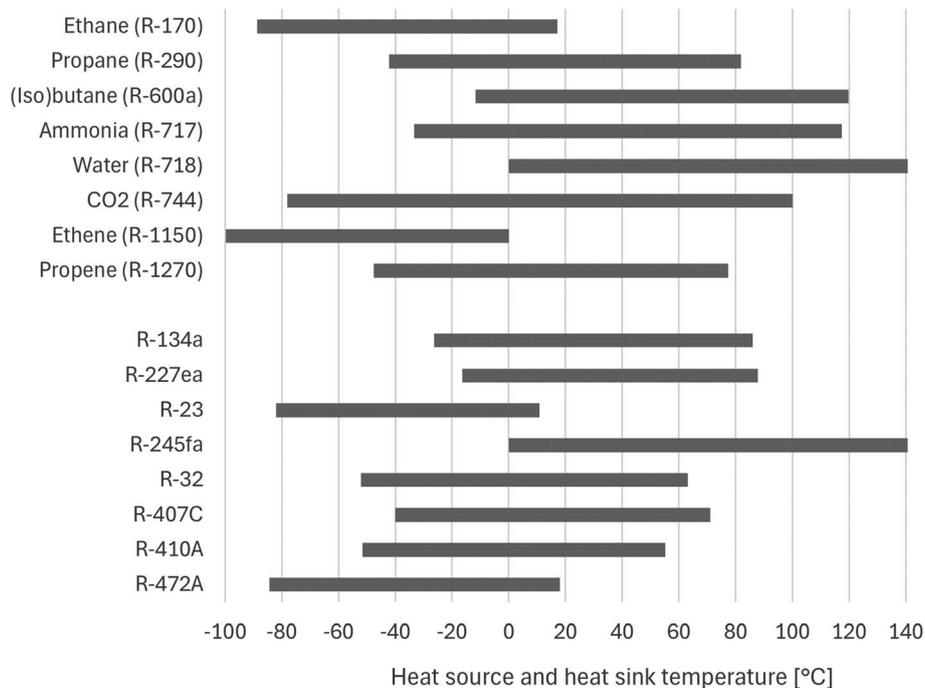
**Fig. 1** Application range of some of the fluorinated and some of the non-fluorinated refrigerants. The lower limit is the normal boiling point, the upper limit is the temperature 15 °C below the substance's critical temperature. Exceptions are R-744 and R-718. Graphic is cut at -100 °C and 140 °C. Adapted from IEA [2020].<sup>39</sup>
