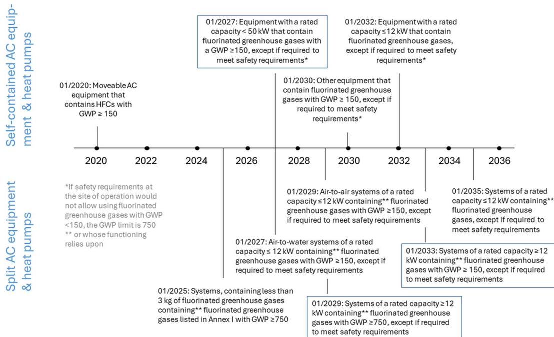
Fig. 3 Placing-on-the-market prohibitions from Annex IV of the F-gas Regulation<sup>9</sup> that refer to self-contained air conditioning (AC) equipment and heat pumps, except chillers (upper part), and split AC equipment and heat pumps (lower part). The blue boxes indicate systems with a rated capacity  $\geq 12$  kW.
