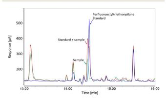
Fig. 1 Comparison of GC-ECD chromatograms for an authentic standard of perfluorooctyl triethoxysilane (blue trace), concealer extract (green trace), and the concealer extract fortified with an authentic standard of perfluorooctyl triethoxysilane (red trace).
