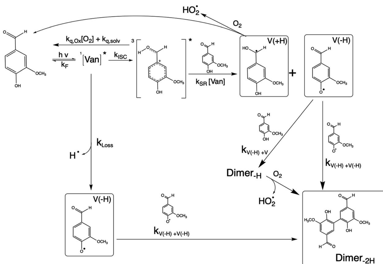
**Scheme 1** Mechanism for photochemical loss of vanillin. Radical propagation through reaction of excited triplet state vanillin with ground state vanillin as well as direct loss of a hydrogen atom lead to a dimer product.
