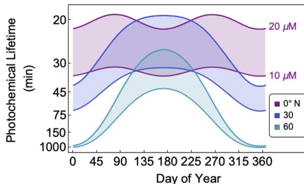
Fig. 6 Effective photochemical lifetime (*e*-folding time) for vanillin using peak daily solar intensity over the course of a year for latitudes spanning  $0^\circ\text{N}$  to  $60^\circ\text{N}$ . Shaded regions indicate the range of lifetimes for  $10 \mu\text{M} < [\text{Van}] < 20 \mu\text{M}$ . Lifetimes are for atmospheric water at  $\text{pH} = 2$  and  $I \sim 0.02 \text{ M}$ .
