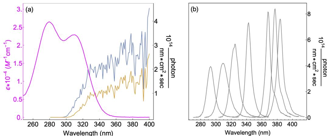
Fig. 1 (a) Base-e molar absorptivity,  $\epsilon$ , of vanillin (magenta), and solar irradiance at 0° (blue) and 60° (yellow) SZA. Solar spectrum data were obtained from the NCAR TUV Model (ozone: 300 DU, albedo: 0.1).<sup>16</sup> (b) LED irradiance source profiles for nominal wavelengths of 295 nm, 310 nm, 325 nm, 340 nm, 365 nm, 375 nm, 385 nm. LED peak irradiance varied by experiment in the range of  $3\text{--}9 \times 10^{14}$  photon per  $\text{nm}^2 \text{cm}^2 \text{sec}$ .
