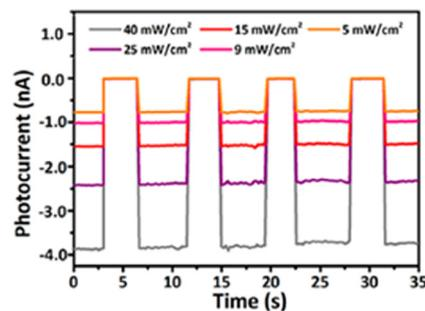
Fig. 32 Photocurrent densities at various incident light intensities of the  $MAPbI_3/(R-4-Br-MBA)_2PbI_4$  device at 785 nm under zero bias. Reprinted with permission from ref. 55 Copyright©2021 American Chemical Society.
