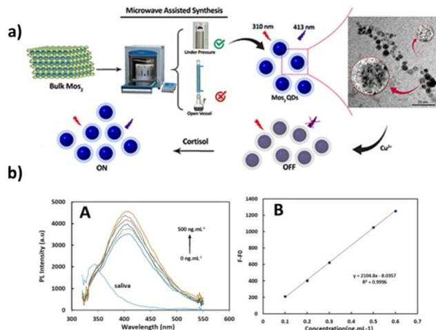
**Fig. 5** (a) Schematic representation of the production of highly luminescent MoS<sub>2</sub> quantum dots (QDs) by microwave exfoliation of the MoS<sub>2</sub> powder. (b) Fluorescence spectra of the MoS<sub>2</sub> QDs–Cu<sup>2+</sup> on cortisol addition in the range of 0–500 ng mL<sup>−1</sup> (left), and calibration curve for cortisol ( $\lambda_{\text{ex}} = 310$  nm and  $\lambda_{\text{em}} = 413$  nm) (right). Adapted from ref. 72 with permission from Elsevier, copyright 2022.
