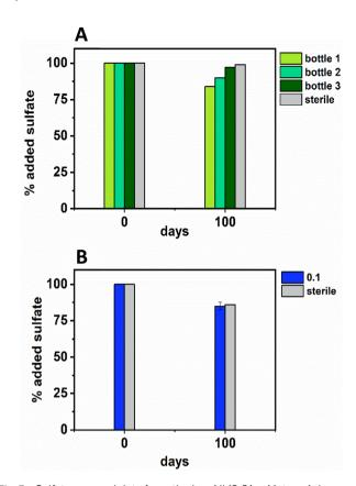
Fig. 3 Sulfate removal data from the low Ni (0.01 mM; top, A, in green) and middle Ni (0.1 mM; bottom, B, in blue) showing the percentage removal by the experimental end point at day 100. For the low Ni experiment (green) each bottle of the triplicate is plotted (due to high variability in between bottles in the triplicate experiment), and, for the middle Ni experiment the average  $\pm\,1\sigma$  is plotted.
