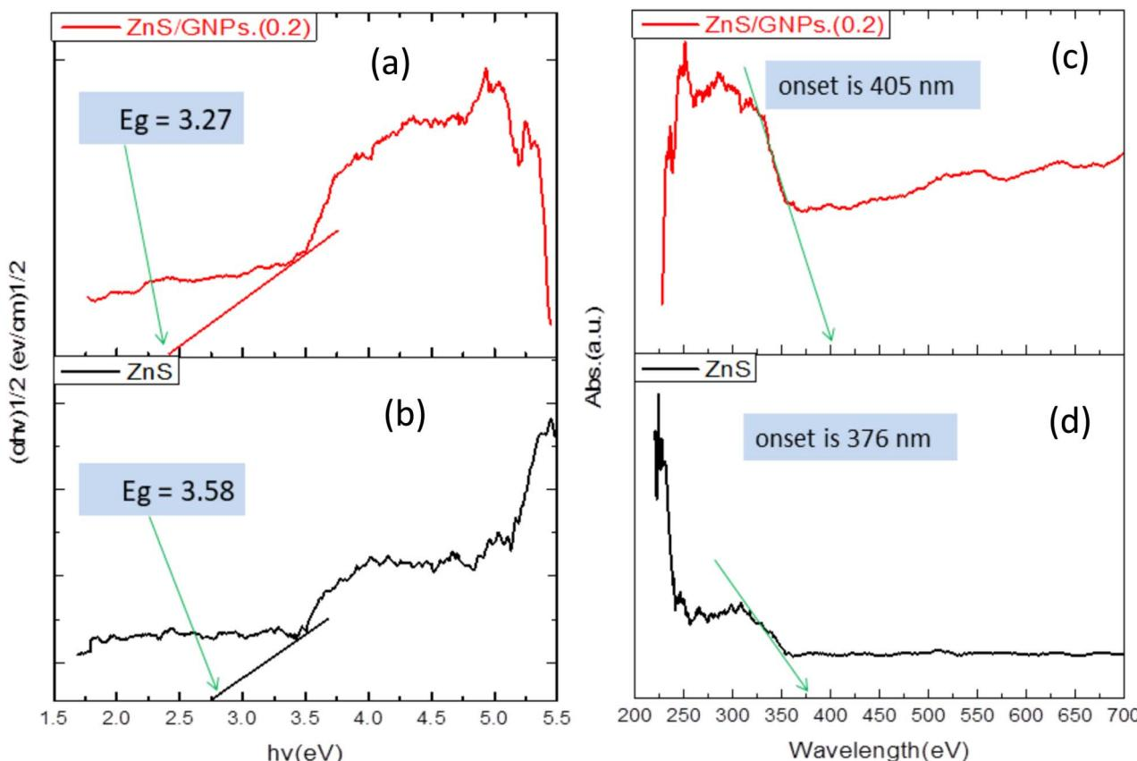
Fig. 6 Band gaps of ZnS/G NPs (a) and ZnS (b); and diffuse reflectance spectra of ZnS/G NPs (c) and ZnS (d), respectively.<sup>53</sup>
