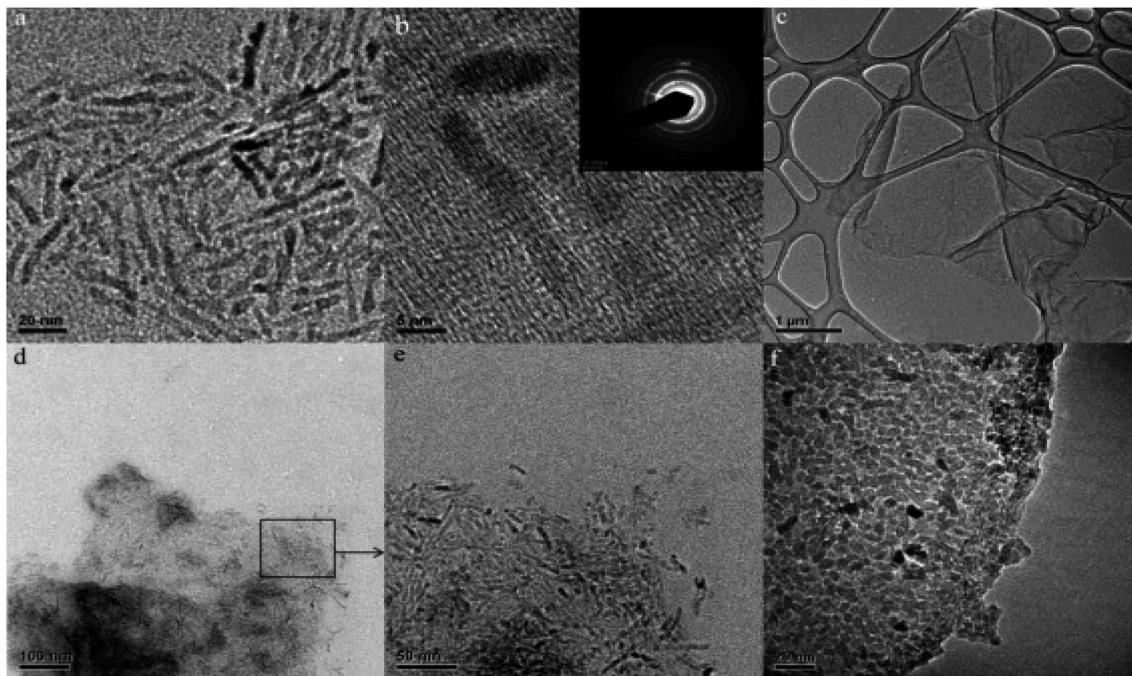
Fig. 5 TEM images of (a) TiO<sub>2</sub> NRs; (b) HRTEM and SEAD of TiO<sub>2</sub> NRs; (c) GO; (d) TiO<sub>2</sub> NRs anchored on GO sheets; (e) enlargement of image d; and (f) TiO<sub>2</sub> NPs anchored on GO sheets reprinted with permission from ref. 67. Copyright 2022 Elsevier.
