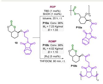
Scheme 3 Synthesis of polymers P10a and P10b
