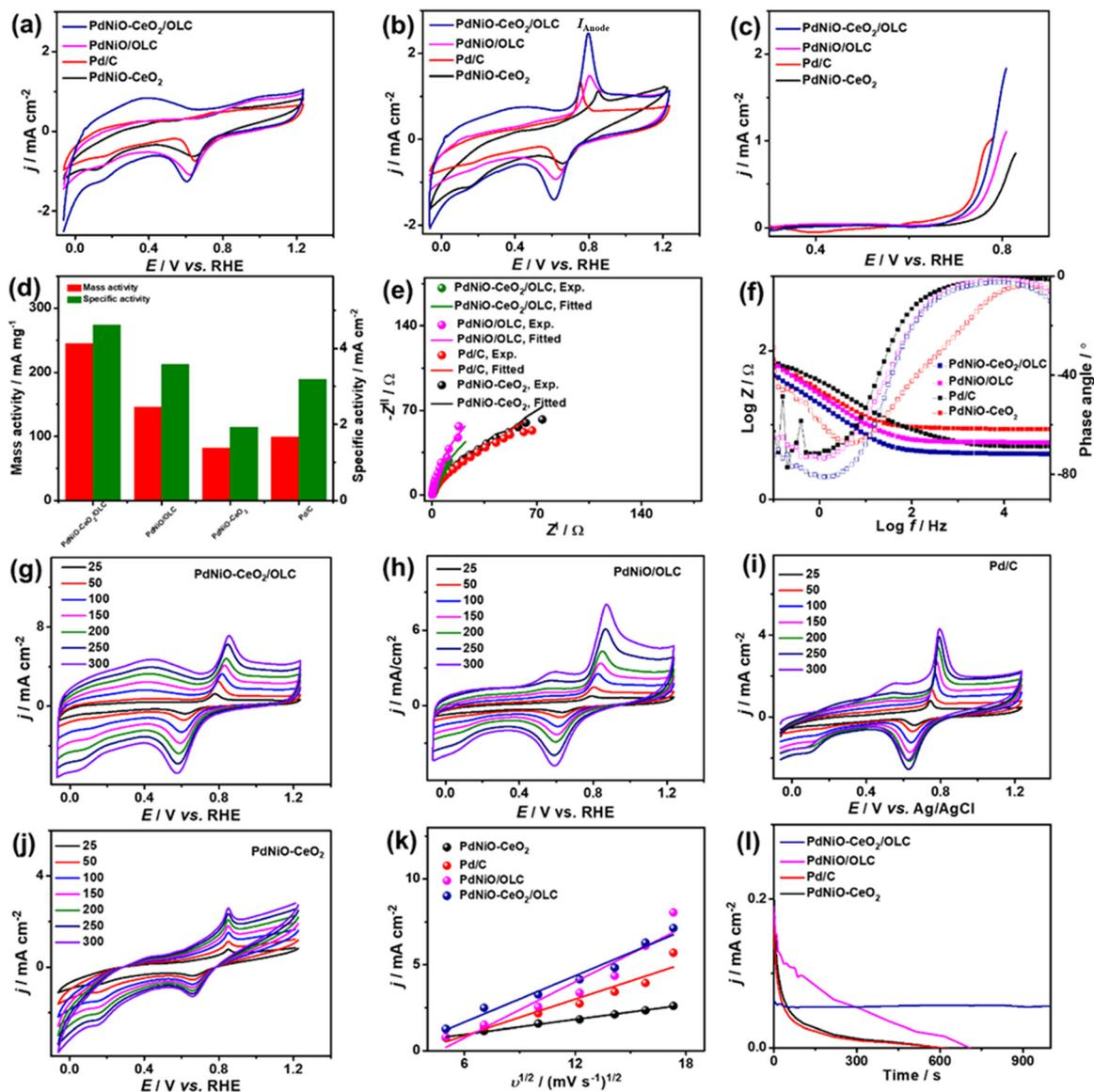
Fig. 4 CV curves at  $50 \text{ mV s}^{-1}$  in (a)  $\text{N}_2$ -saturated KOH (0.1 M) and (b) CO-saturated KOH (0.1 M). (c) LSV at  $50 \text{ mV s}^{-1}$ . (d) Mass/specific activities. (e) Nyquist plots. (f) Bode plots. (g–j) Scan rate studies. (k) Randles-Sevcik plots ( $I_{\text{Anode}}$  vs.  $v^{1/2}$ ) and (l) CA of PdNiO-CeO<sub>2</sub>/OLC, PdNiO/OLC, PdNiO-CeO<sub>2</sub>, and Pd/C in CO-saturated KOH (0.1 M).
