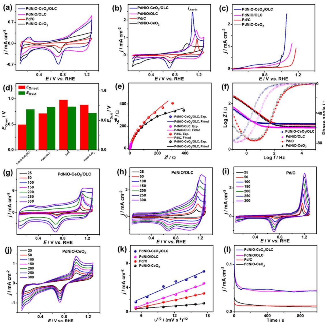
Fig. 3 CV profiles at  $50 \text{ mV s}^{-1}$  in (a) N<sub>2</sub>-saturated HClO<sub>4</sub> (0.1 M) and (b) CO-saturated HClO<sub>4</sub> (0.1 M). (c) LSV at  $50 \text{ mV s}^{-1}$ . (d)  $E_{\text{Onset}}$  and  $E_{\text{Oxid}}$ . (e) Nyquist plots. (f) Bode plots. (g–j) Scan rate studies. (k) Randles-Sevcik plots ( $J_{\text{Anode}}$  vs.  $v^{1/2}$ ). (l) CA of PdNiO-CeO<sub>2</sub>/OLC, PdNiO/OLC, PdNiO-CeO<sub>2</sub>, and Pd/C in CO-saturated HClO<sub>4</sub> (0.1 M).
