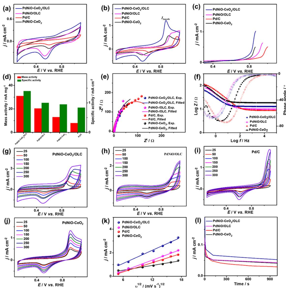
Fig. 5 CV profiles at 50 mV s<sup>-1</sup> in (a) N<sub>2</sub>-saturated NaHCO<sub>3</sub> (0.1 M) and (b) CO-saturated NaHCO<sub>3</sub> (0.1 M). (c) LSV at 50 mV s<sup>-1</sup>. (d) Mass/specific activities. (e) Nyquist plots. (f) Bode plots. (g–j) Scan rate studies. (k) Randles–Sevcik plots ( $I_{\text{Anode}}$  vs.  $v^{1/2}$ ) and (l) CA of PdNiO–CeO<sub>2</sub>/OLC, PdNiO/OLC, PdNiO–CeO<sub>2</sub>, and Pd/C in CO-saturated NaHCO<sub>3</sub> (0.1 M).
