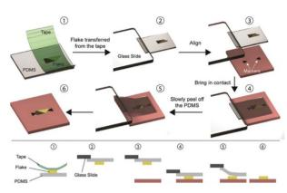
Fig. 3 The PDMS dry transfer method. The flake to be transferred is exfoliated onto a PDMS stamp (1) and the stamp is then attached to a glass slide connected to a micromanipulator (2). Using a microscope, the flake can be aligned with the final substrate (3) and brought into contact (4). By slowly peeling the PDMS stamp (5) the flake can be deposited on the substrate (6). Reproduced from ref. 81 with permission from Royal Society of Chemistry (RSC), copyright 2020.
