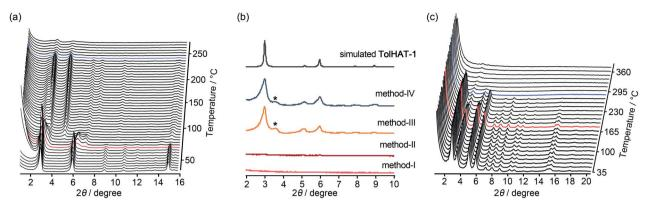
Fig. 5 (a) Variable temperature (VT)-PXRD patterns of the as-formed HOF TolHAT-1. (b) PXRD patterns of activated HOF TolHAT-1aN (N = I - IV) with the simulation pattern of TolHAT-1. (c) VT-PXRD patterns of TolHAT-1aIV from rt to 360 °C. Red line indicates the temperature where the network begins to collapse and blue line corresponds to the temperature where the framework is fully collapsed. The asterisk (\*) denotes a non-identifiable peak appeared for the activated TolHAT samples.
