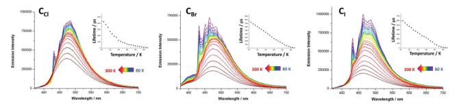
Fig. 3 Temperature dependence (80 K to 300 K) of the solid-state emission spectra of metallacycles C<sub>CI</sub>, C<sub>Br</sub> and C<sub>I</sub> upon excitation at 325 nm.‡ Inset: plot of their emission decay lifetime against temperature (80 K to 300 K).
