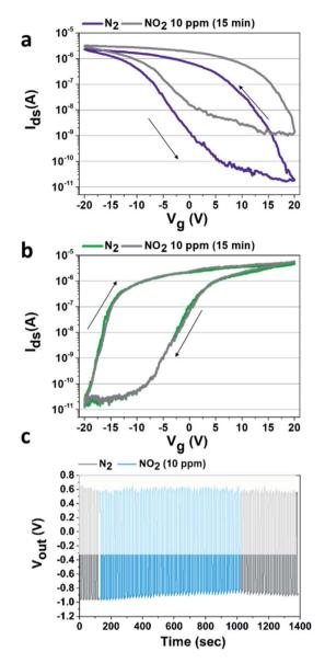
Fig. 2 (a)  $I_{\rm ds}-V_{\rm g}$  characteristic of the p-type SWCNT-FET before and after 15 min of NO<sub>2</sub> exposure ( $V_{\rm DS}=1$  V). (b)  $I_{\rm ds}-V_{\rm g}$  characteristic of the n-type SWCNT-FET before and after 15 min of NO<sub>2</sub> exposure ( $V_{\rm DS}=-1$  V). (c) Output voltage as a function of time of the inverter under an exposure of NO<sub>2</sub> gas for a square input voltage for alternatively -4 V and -11 V ( $V_{\rm DD}=2$  V).
