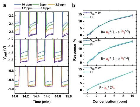
Fig. 3 (a) Output voltage of the inverter after exposure to various concentrations of  $NO_2$  gas for a  $V_{in}$  at -4 V and -11 V alternatively for three different  $V_{DD}$  values (from top to bottom:  $V_{DD} = 6 \text{ V}$ , 4 V and 2 V). (b) Response of the inverter as a function of NO<sub>2</sub> concentration for the three different  $V_{\rm DD}$  values (from top to bottom:  $V_{\rm DD} = 6$  V, 4 V and 2 V).
