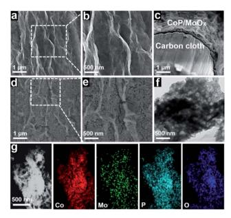
Fig. 2 (a and b) SEM image and magnified SEM image of  $CoP/MoO_x$  thin films. (c) SEM image of the cut surface of  $CoP/MoO_x$  thin films. (d and e) SEM images of porous  $CoP/MoO_2$  thin films. (f) TEM image of a typical porous  $CoP/MoO_2$  thin film. (g) HAADF-STEM image and elemental mapping images of Co, Mo, P and O in the porous  $CoP/MoO_2$  thin films.
