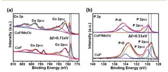
Fig. 1 XPS spectra of porous CoP/MoO<sub>2</sub> thin films and pure CoP thin films: (a) Co 2p spectra, (b) P 2p spectra.
