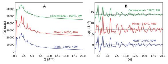
Fig. 3 (A) Raw total scattering data, I(Q), for the conventional (green), mixed MWR-conventional (red) and MWR-only (blue) synthesis conditions. Sharper peaks are present in the final product for MWR-grown samples. (B) PDF data, G(r), for the same datasets as in (A). The increase in Bragg intensity shown in (A) is found to be due to an increase in particle size, as seen by the increase in intensity of peaks at higher r values for samples grown by MWR-assisted synthesis.
