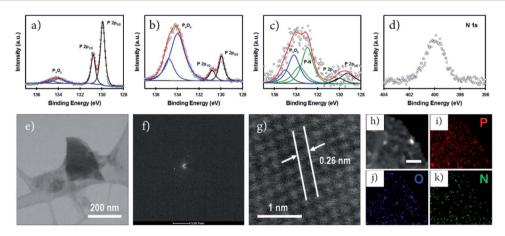
Fig. 2 High resolution P 2p XPS spectra of (a) non-doped, (b) O-doped, and (c) N-doped phosphorene nanosheets. (d) N 1s XPS spectrum, (e) TEM image, (f) SAED pattern and (g) HRTEM image of the N-phosphorene. (h) High-angle annular dark-field-scanning transmission electron microscope (HAADF-STEM) image of an N-phosphorene nanosheet (scale bar: 50 nm), and (i-k) the corresponding EDX elemental mapping images.
