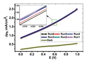
Fig. 7 Reproducible studies of photocurrent density—voltage curves of the PbS-Cr6 electrode in dark and under white light illumination without the optical filter.
