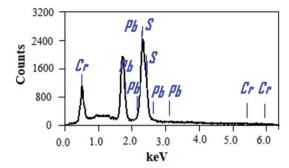
Fig. 2 EDX spectrum of PbS-6Cr film.
