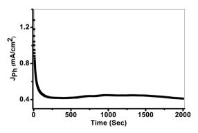
Fig. 8 Current-time characteristic under white light illumination.
