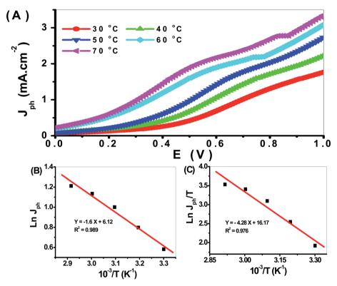
Fig. 11 (A) The effect of temperature on  $H_2$  generation process, (B) plot of the  $J_{ph}$  against reciprocal of temperature, and (C) plot of  $J_{ph}/T$  versus reciprocal of reciprocal temperature.
