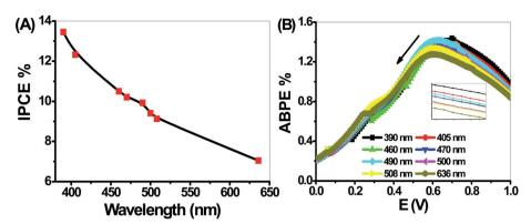
Fig. 10 (A) IPCE% and (B) ABPE% as a function of wavelength for the PbS-Cr6 electrode.
