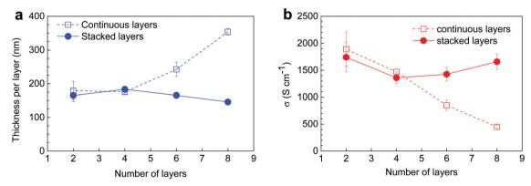
Fig. 2 (a) Evolution of the thickness per layer and (b) electrical conductivity as a function of the number of layers for PEDOT:OTf films polymerized with 5 wt% NMP, for continuous layers (empty squares) or stacked layers (full rounds).
