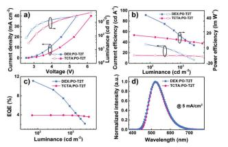
Fig. 4 (a) J-V-L plots, (b) CE-luminance-PE plots, (c) EQE-luminance plots, and (d) EL (at 5 mA cm<sup>-2</sup>) spectra of **DEX:PO-T2T** and TCTA:**PO-T2T** exciplex-based devices.
