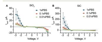
Fig. 4 Gate leakage current. Gate leakage current at different solution concentrations for SiO<sub>2</sub> dielectric layer (A) and SiC dielectric layer (B).
