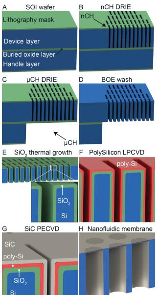
Fig. 1 Fabrication process schematics A) Silicon on insulator (SOI) wafer with lithography mask B) deep reactive ion etching (DRIE) for nanochannel (nCH) patterning. C) DRIE for microchannel ( $\mu$ CH) pattern. D) SiO<sub>2</sub> mask removal. E) SiO<sub>2</sub> thermal oxidation growth. F) Conductive poly-Si deposition. G) Insulating SiC deposition. H) Membrane structure
