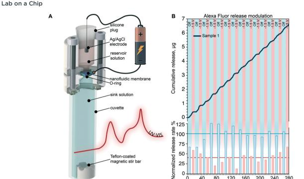
Fig. 6 Modulated release of Alexa Fluor 647. A) Rendering of custom device used for *in vitro* release rate modulation. B) *In vitro* cumulative release modulation of Alexa Fluor (top). Release rate for every phase, normalized to the average of the passive phases. Blue and red line represent the average of the passive and active (–1.5 V) phases respectively.
