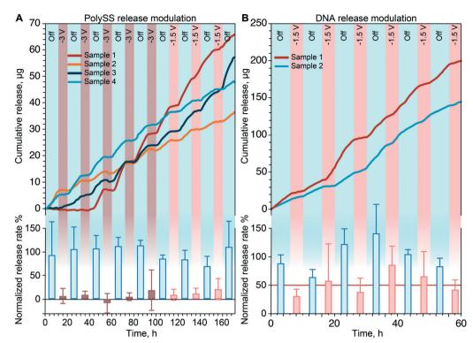
Fig. 7 Modulated release of poly(sodium 4-styrenesulfonate). A) In vitro cumulative release modulation of polySS (top). Release rate for every phase, normalized to the average of the passive phases (bottom). B) In vitro cumulative release modulation of DNA (top). Release rate for every phase, normalized to the average of the passive phases. Red line represents the average of the active (-1.5 V) phases.
