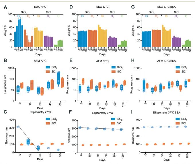
Fig. 3 Nanofluidic membrane degradation. Energy-dispersive X-ray spectroscopy (EDX) for membranes coated with SiO2 versus SiC at 77 °C (A), 37 °C (D) and at 37 °C with BSA (G). Surface roughness calculated with atomic force microscopy (AFM) for membranes coated with SiO<sub>2</sub> versus SiC at 77 °C (B), 37 °C (E) and at 37 °C with BSA (H). Layer thicknesses fitted through ellipsometry data for membranes coated with SiO<sub>2</sub> versus SiC at 77 °C (C), 37 °C (F) and at 37 °C with BSA (I).
